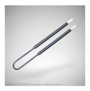
MolyCom®-Ultra and MolyCom®-Hyper electric heating elements are metallic-ceramic materials mainly composed of molybdenum disilicide (MoSi<sub>2</sub>). Above 1.000 °C service temperature the surface will form a protective high-temperature layer of pure quartz, which gives the MolyCom® heating elements a high resistance to oxidation.
