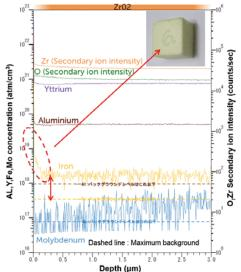
Fig. 7: Secondary ion mass spectrometry (SIMS) of a contaminated ZrO<sub>2</sub> sample.
