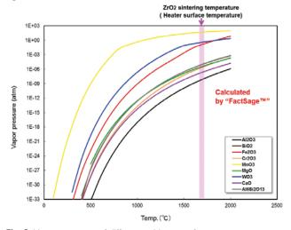
**Fig. 8:** Vapor pressures of different oxides at surface temperatures of heating elements in use.
