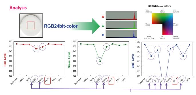
Fig. 4: Proof of the color change by RGB 24 Bit color colorimeter.
