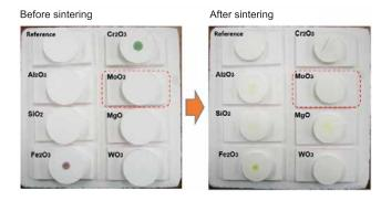
Fig. 3: Test with several oxides on ZrO<sub>2</sub>-samples.
