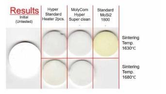
Fig. 5: Color changes from different heating element qualities.
