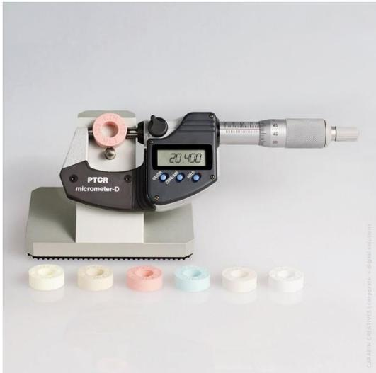
For precise determination of the shrinkage of a process temperature control ring PTCR, a precise and even measurement is decisive. To ensure this, we offer a special digital **micrometer** with precise holder for the rings and a USB interface for data transmission. A specifically developed holder ensures reproducible positioning of the PTCR in the **micrometer**.
